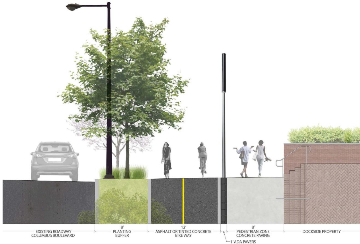
FIGURE 1. DRT On-Road - Typical Section – Dockside Residences
